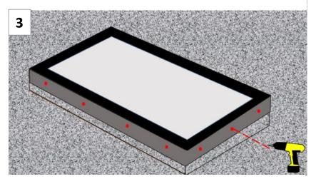
Pre drill fixing holes through aluminium and timber upstand/kerb at 100mm from each corner, and then at regular intervals all around.
