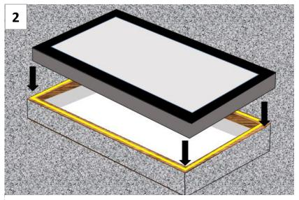
Position the framed fixed Infinity Rooflight over the top and the side of the upstand/kerb.
