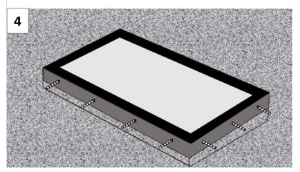
Secure fixing screws with horse shoe packers and finishing caps continuously all the way around, securing the Infinity Rooflight in place.
