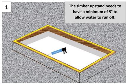
Apply a thick bead of silicone all the way around on top of the timber upstand/kerb.
